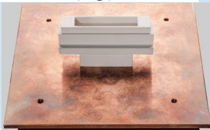
Right: early 3D-printed antenna prototype
